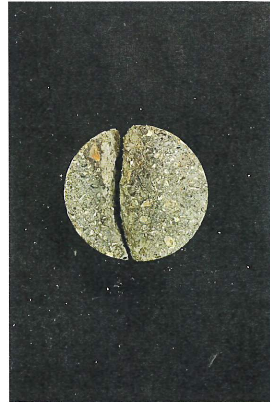
TH #3 Top of Asphalt Pavement Ø = 150 mm
