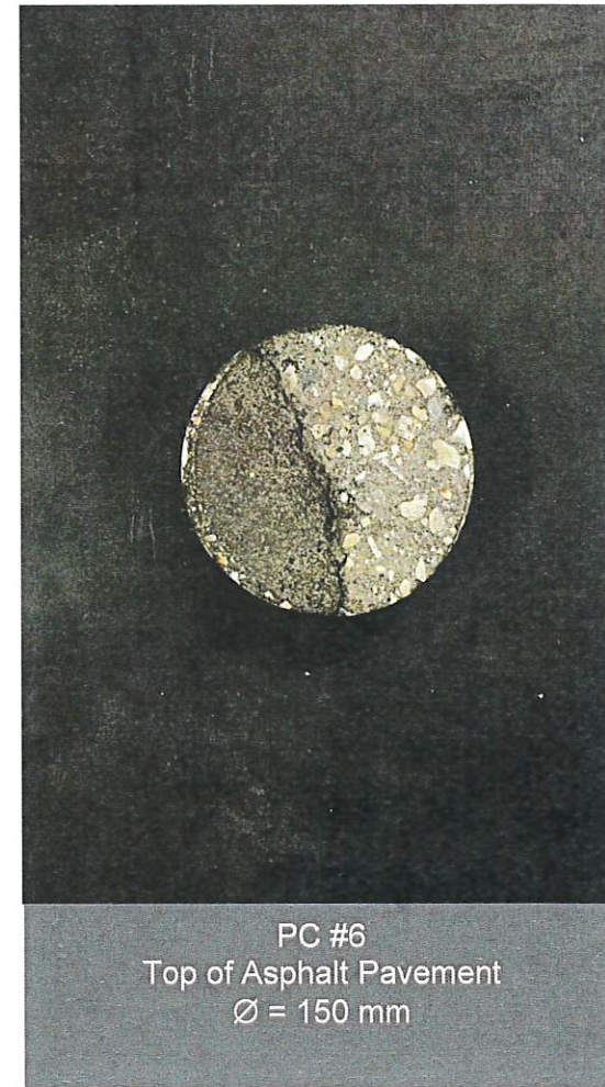
Photograph 6: Specimen from Bishop Grandin Boulevard, Westbound Lane Longitudinal Joint between Lanes
